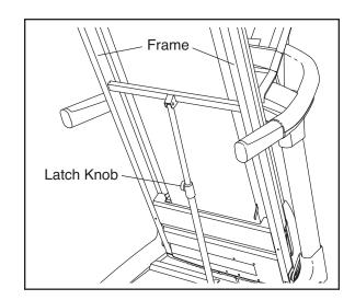
Hold the metal frame firmly with both hands, and lower it to the floor. CAUTION: To decrease the possibility of injury, do not lower the frame by gripping only the plastic foot rails. Do not drop the frame to the floor. Make sure to bend your legs and keep your back straight.
